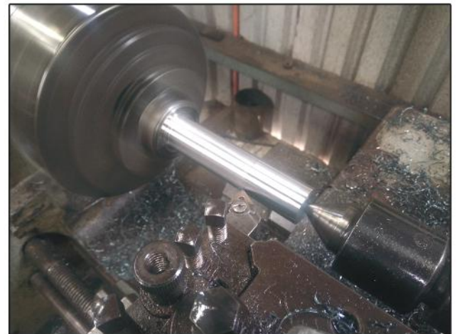
The first pin for the tender bogie suspension being machined in-house on the lathe
